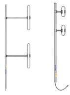
The SD242 series is an extremely rugged 2-bay exposed dipole antenna designed for applications where moderate gain is required and Passive Intermodulation interference (PIM) is a consideration. These premium-quality antennas are well suited for public safety applications. The design of these antennas provides for coverage from 118 to 225 MHz in 3 sub bands, the 138-174 MHz band is for private mobile networks and public safety.
