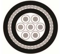
APPLICATION: For Mains and Sub Mains Control Circuits requiring Mechanical Protection,
